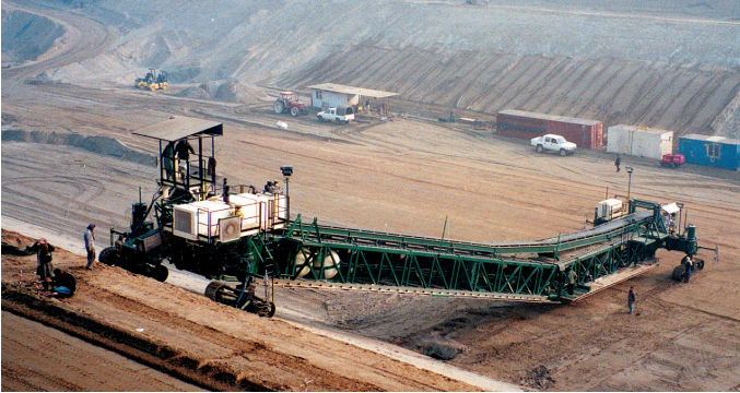
Half Span Liner walking up the slope under its own power.
